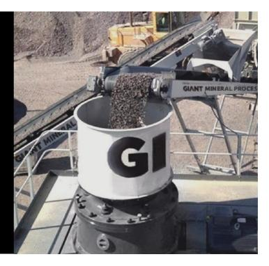
The crusher setting is instantaneously maintained even after passing a piece of tramp iron.
